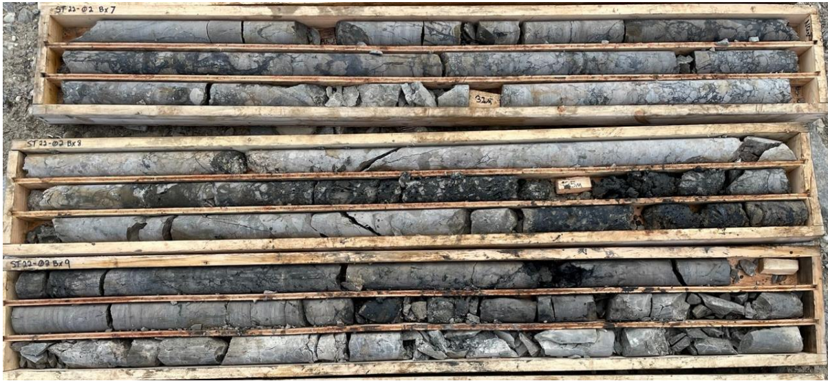
Figure 3: Sooty sulfides within fractured dolomite in drill hole ST22-01 (approx. 29m – 38.31m downhole).
