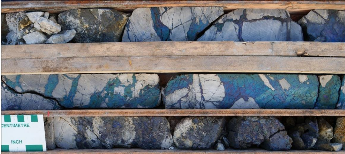
Figure 1: Massive and fracture-fill bornite and chalcocite from approx. 50m downhole in ST22-05.
