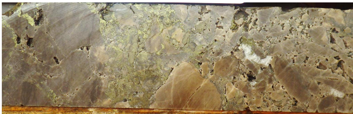
Figure 1: Chalcopyrite (copper sulfide) within ST22-10 drill core from 313m downhole. Chalcopyrite is the metallic yellow mineral within tan/grey dolostone/limestone.
