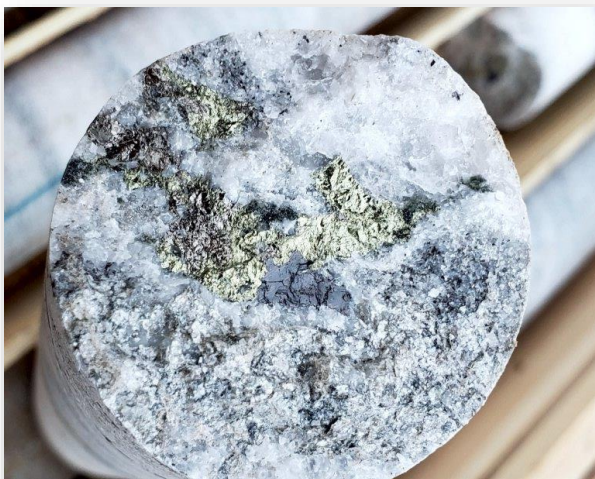
Chalcopyrite and sphalerite in core from October 2021 drilling, Mountain Project
