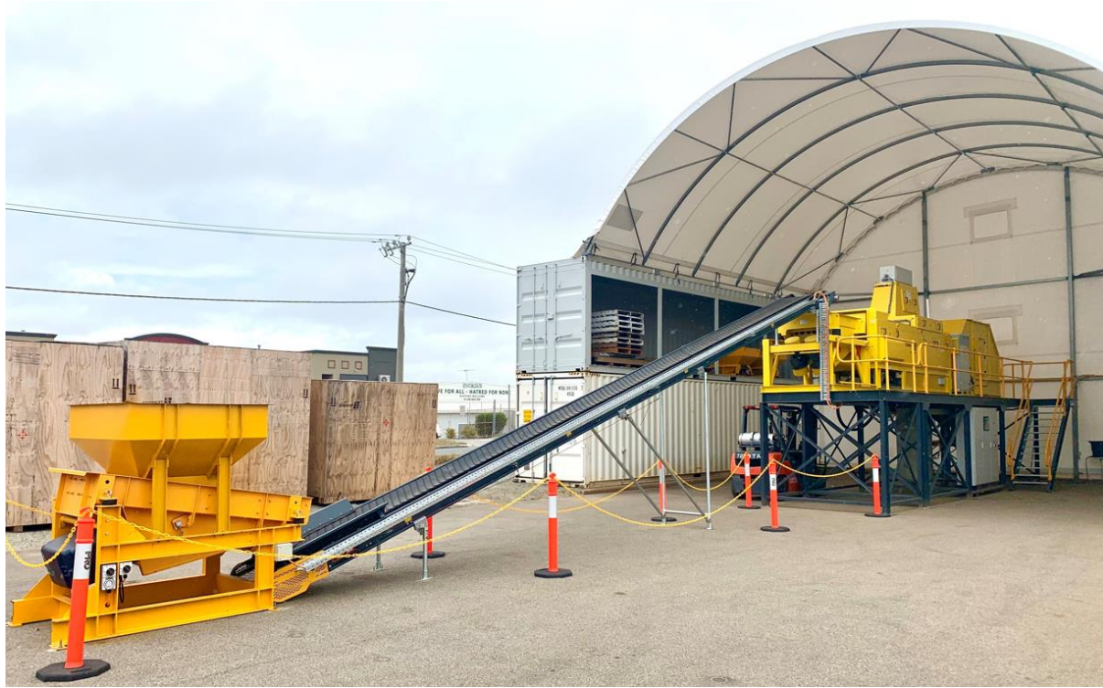
Figure 1: Full scale Steinert KSS ore sorter, Bibra Lake, Western Australia
