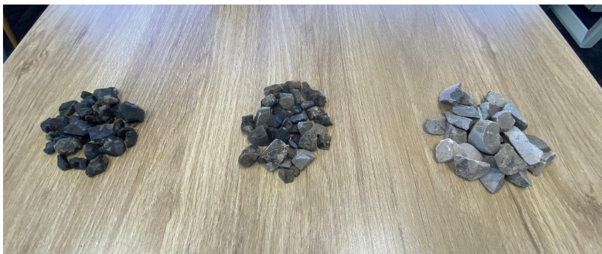
Figure 3: The three products produced from the ore sorting test work. Left to right – very high density product, intermediate product, and low density product (waste rock).
