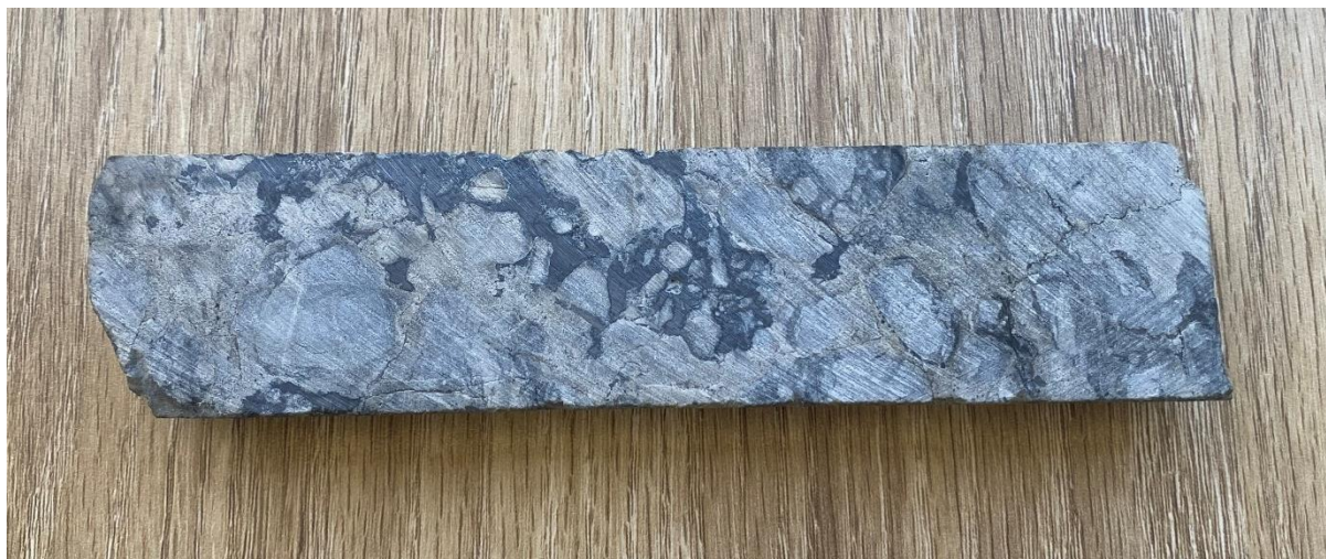
Figure 2: Drill core from STOR1601D from interval 97-101m downhole – average grade 4.16% Cu. The chalcocite is seen as the dark gunmetal grey material within the lighter grey dolomite host rock.
