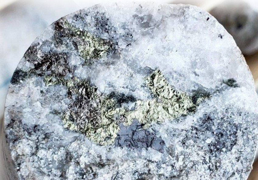
Chalcopryrite and sphalerite in core from October 2021 drilling, Mountain Project
