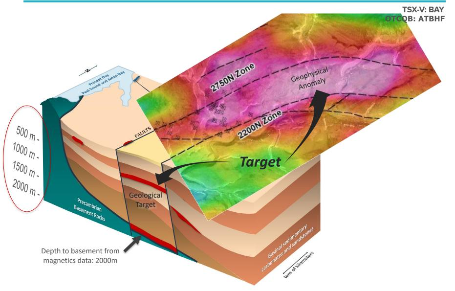
The challenge: deep sedimentary basin + poor depth control with gravity. Additional ground geophysics is planned to identify prospective targets at reasonable depths
