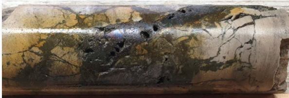
Chalcocite-chalcopyrite mineralization from ST23-03
