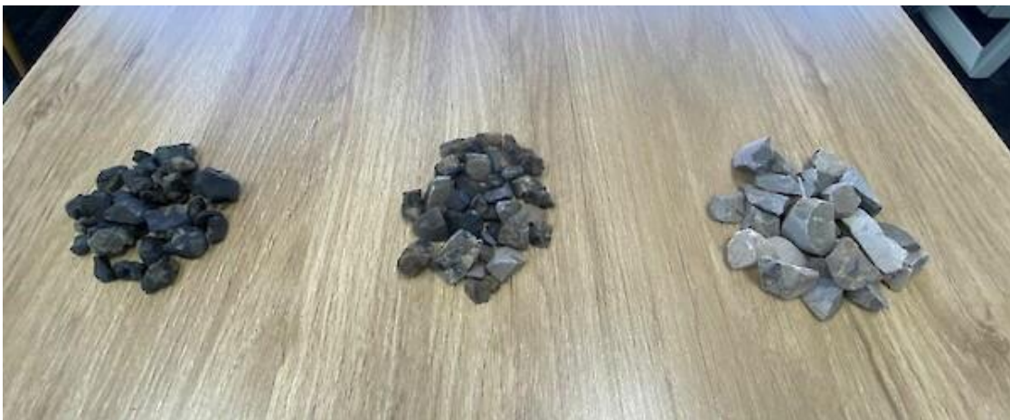
Figure 7: The three products produced from the ore sorting test work. Left to right - very high density product, intermediate product, and low density product (waste rock).
