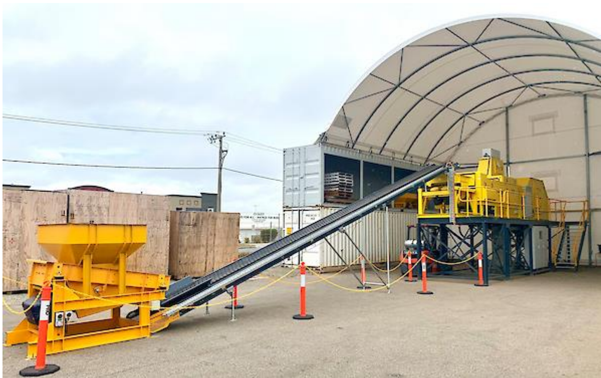
Figure 5: Full scale Steinert KSS ore sorter, Bibra Lake, Western Australia
