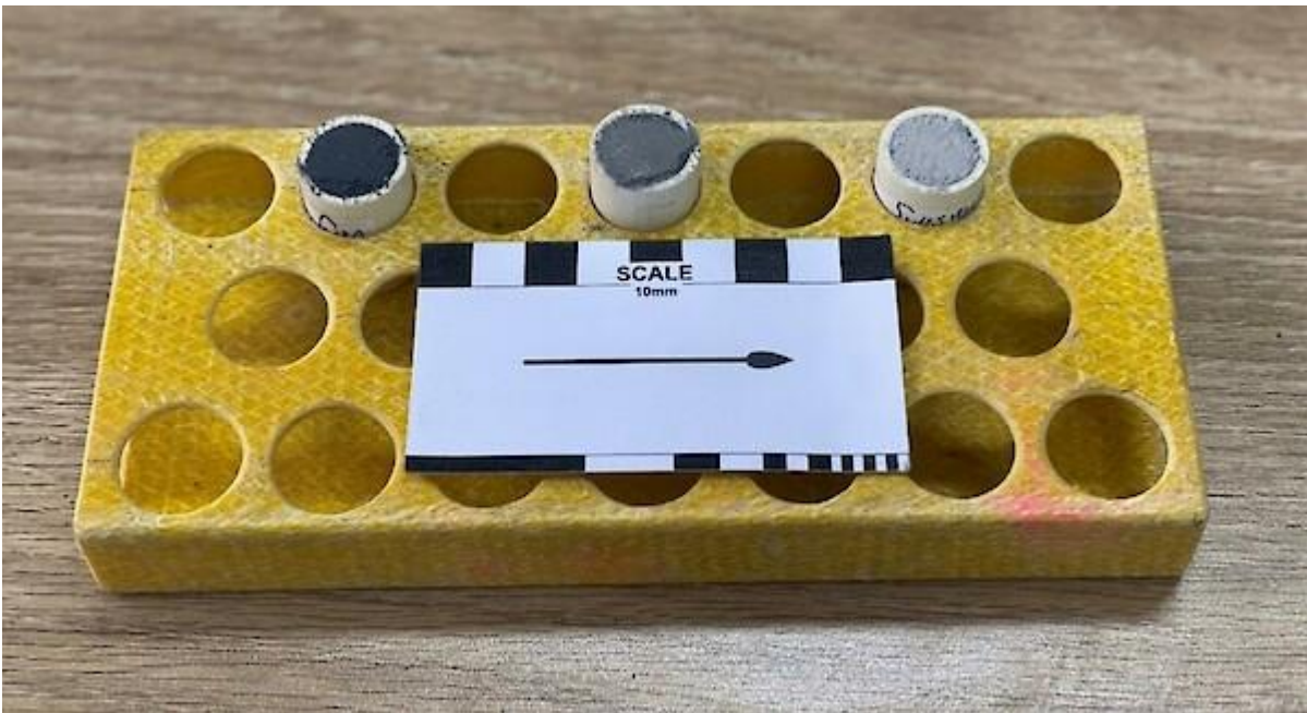
Figure 8: Pressed pellets generated from the ore sorting products ready for XRF analysis.
