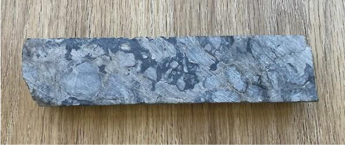
Figure 6: Drill core from STOR1601D from interval 97-101m downhole - average grade 4.16% Cu. The chalcocite is seen as the dark gunmetal grey material within the lighter grey dolomite host rock.
