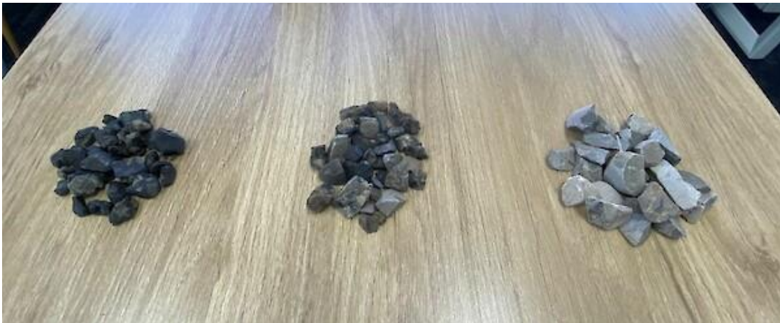
Figure 11: The three products produced from the ore sorting test work. Left to right - very high density product, intermediate product, and low density product (waste rock).
