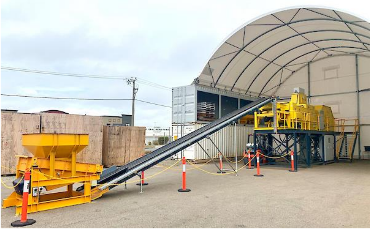
Figure 9: Full scale Steinert KSS ore sorter, Bibra Lake, Western Australia
