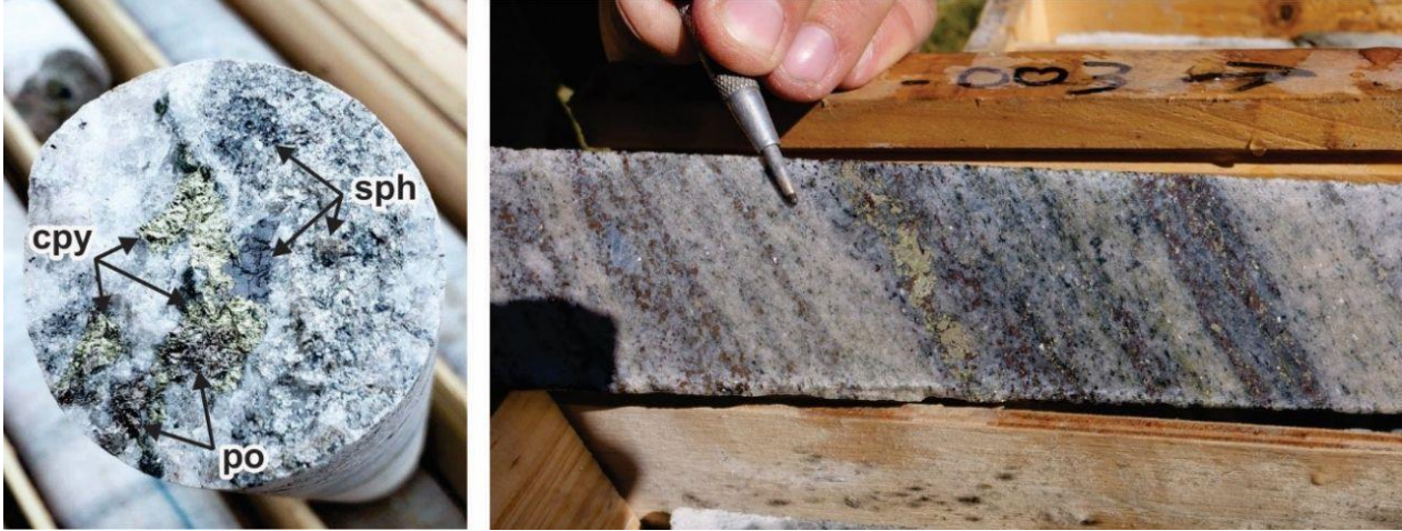
Figure 3: Banded disseminated sulfide mineralization in drill core, Mountain Base Metals Project, Central Virginia (cpy = chalcocopyrite, sph = sphalerite, po = pyrrhotite). Drillhole ABM21-003, approximately 265 meters down hole. Core diameter 47 millimeters (1.8 inches).
